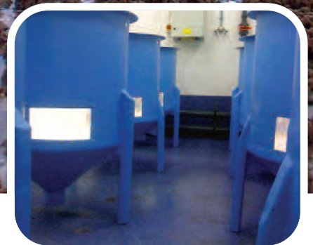
> The paddle VORtex Resuspension Tanks (pVORTs) in the SAMs aquarium is used to generate current flow and continuous suspension of sediment.
