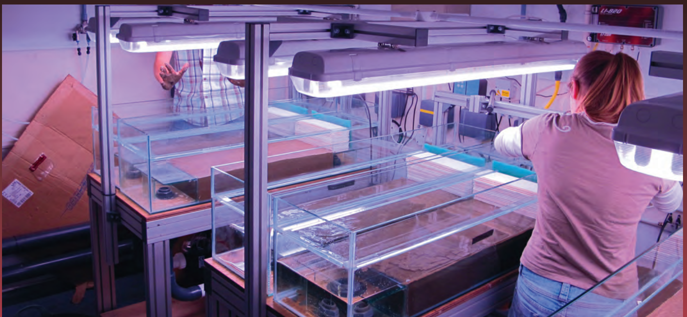
Figure 2: The custom-built flume facility at SAMS is used to study the combined impacts from ocean acidification and temperature increases on benthic biogeochemistry in cohesive mud and in carbonate sand.
